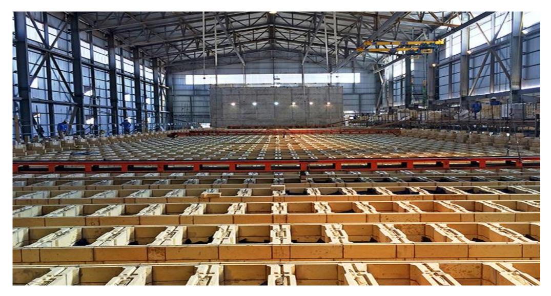
A coke oven battery is a complex structure of many different refractory shapes, but it can be divided in general into two sections; the regenerators which are the lower section, and the coking and combustion chambers which represent the upper section. The refractories used require good mechanical strength, thermal shock resistance abrasion resistance, volume stability, and in the upper section good hot strength.
